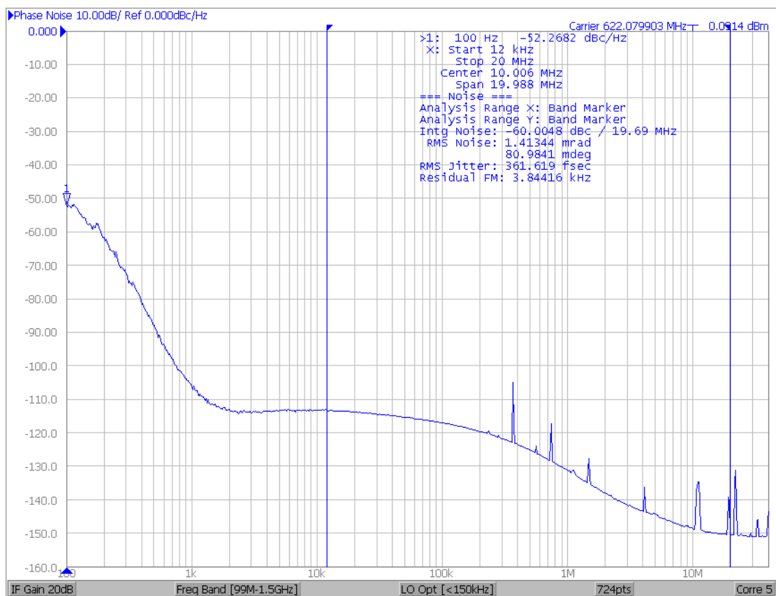
Figure 60. Si5317 at 622.08 MHz with a 40 MHz Crystal
